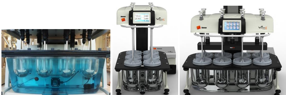
Figure 4 Space between vessel and head (e.g. Hanson SR8, Vision Classic, and Vision Elite)
